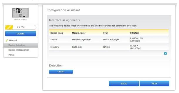
Fig.: Configuration wizard - Example - Interface Assignments
