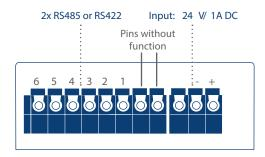
Fig.: Top Connections – Gateway Solar-Log 50
