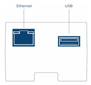
Fig.: Bottom connections Gateway Solar-Log 50
