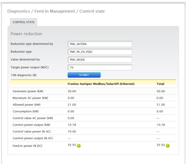
Fig.: Feed-in management – control status example
