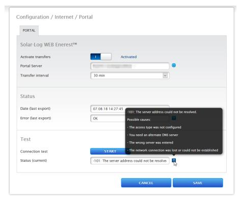
Fig.: Example - Connection Test with an Error
