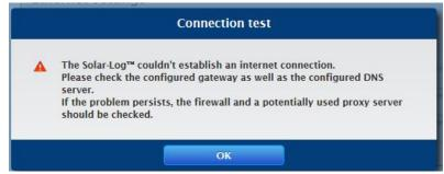
Fig.: Example of an unsuccessful connection test
