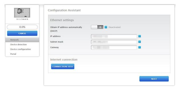
Fig.: Solar-Log™ Ethernet settings from the Solar-Log™ Configuration Wizard
