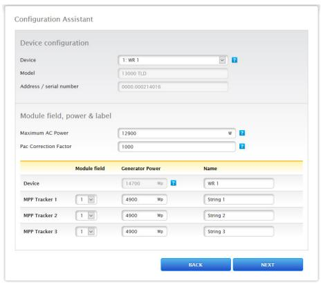
Fig.: Example - Configuration Wizard - Device Configuration
