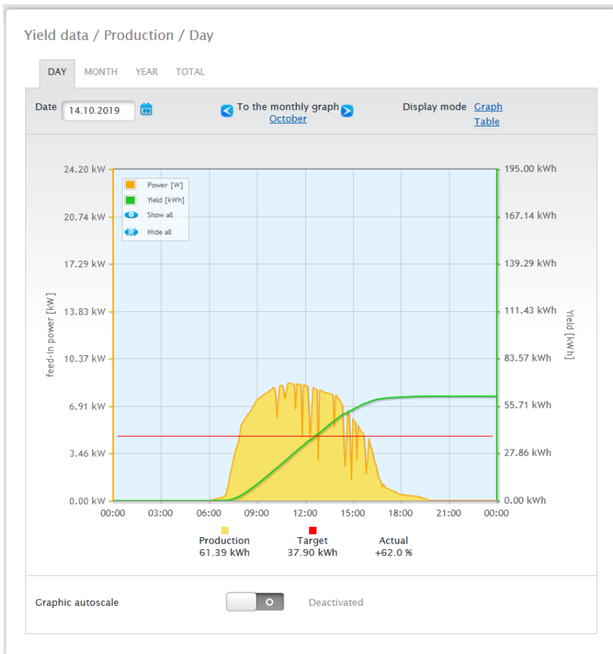
Fig.: Daily View of the Production Graph with the Auto Scaling deactivated
