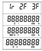
Energy flow direction display per phase 1 2 3 R = Reverse. F = Forward
